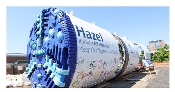
A new 380-ton, 14 feet 8 inches tall tunnel boring machine (TBM) named Hazel has been unveiled by AlexRenew, Alexandria's wastewater authority, marking a significant milestone in its RiverRenew program to improve local waterways.
